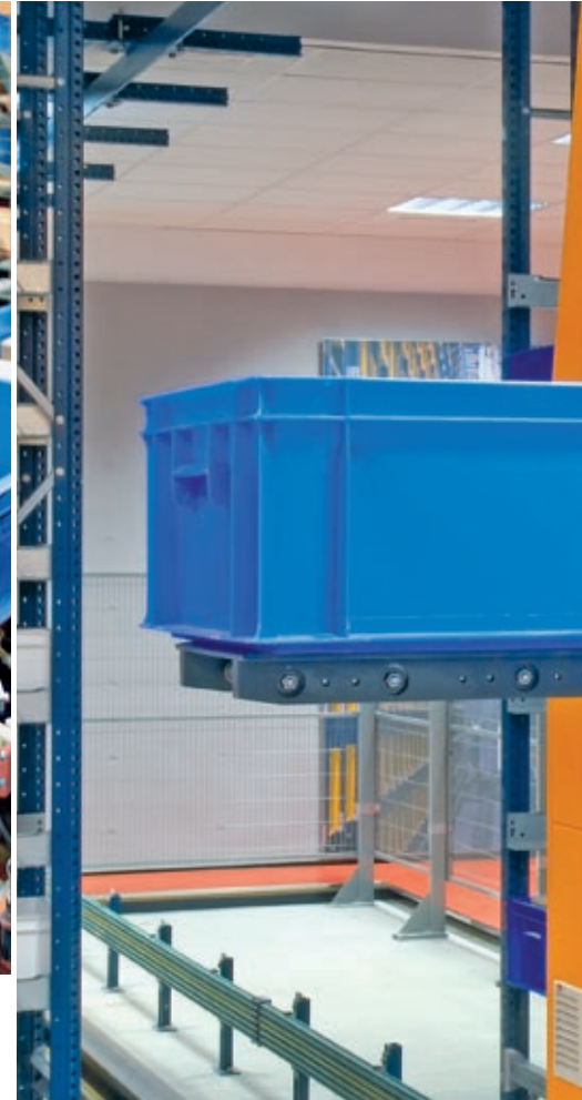
Extraction system with forks to extract two boxes at the same time
