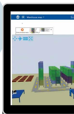
The software uses rules and strategies, applicable to the goods and to the logical structure of the warehouse, that streamline storage tasks performed by operators or machines and provide constant maintenance of the order of products in the warehouse. All this provides perfect stock control in real-time.
