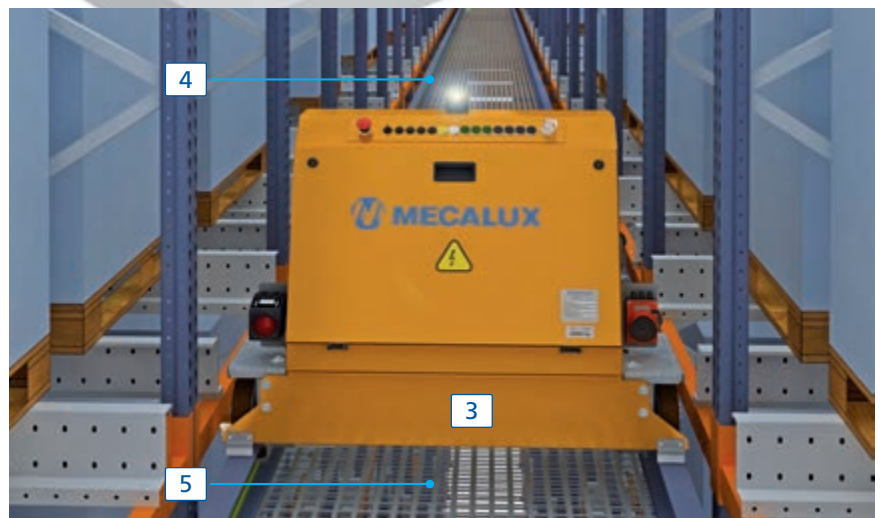
Close-up of the transfer car and the maintenance floor.
