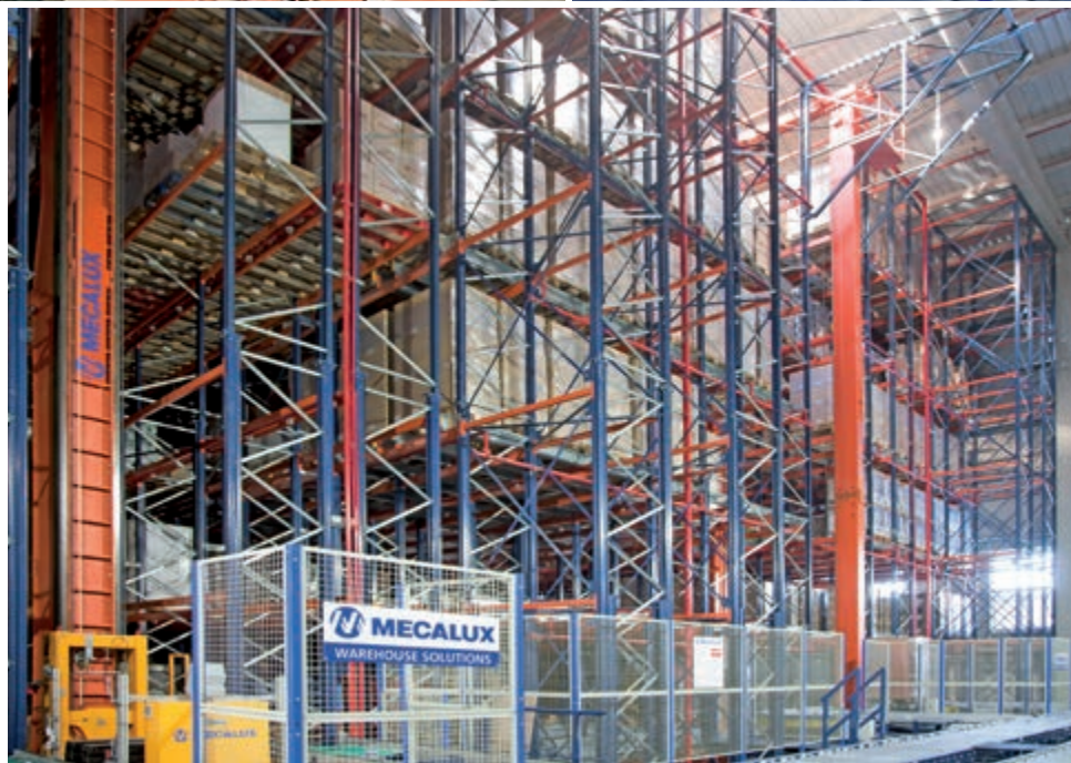
Automated warehouse with automated Pallet Shuttle (3) for picking and automated warehouse with double-depth racking (4).
