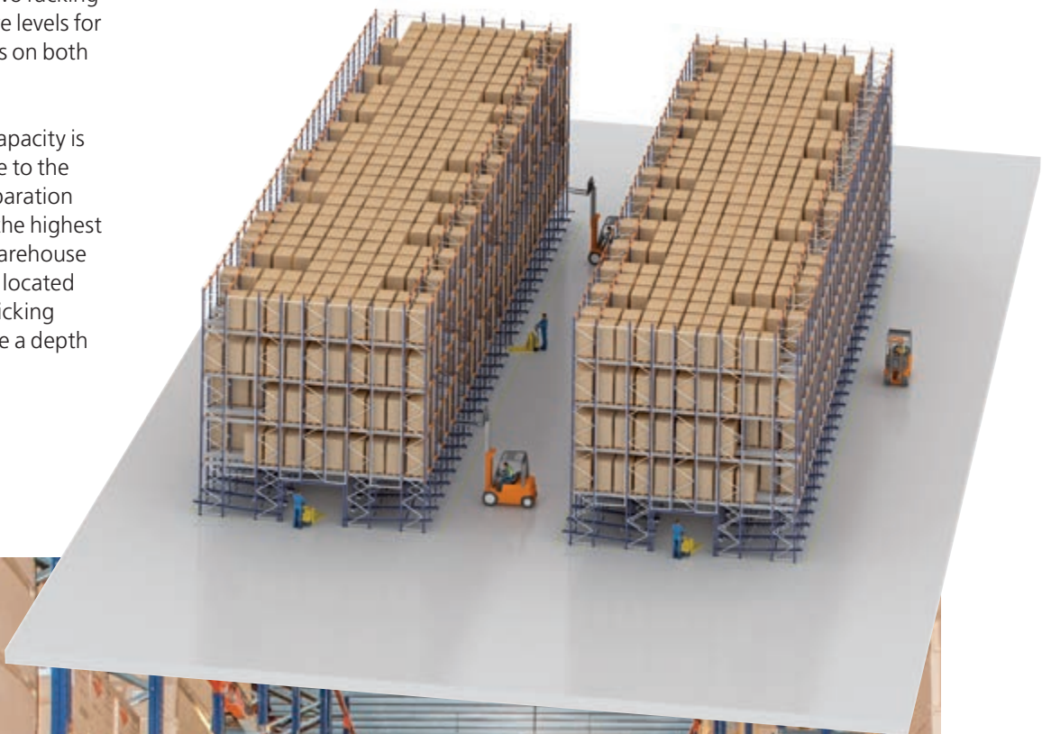
Solution 4. Warehouse with semi-automated Pallet Shuttle system consisting of two modules combined with live levels for picking.
