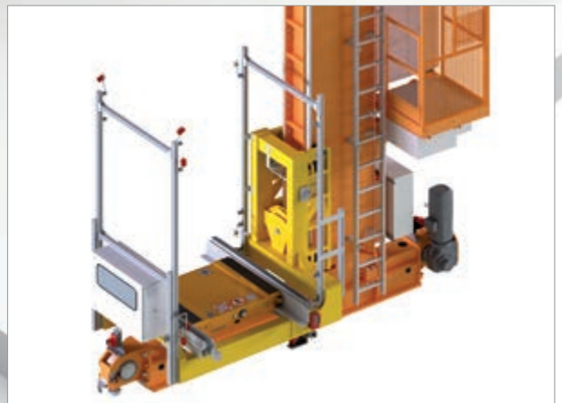
Close-up of Pallet Shuttle in the cradle of the stacker crane.
