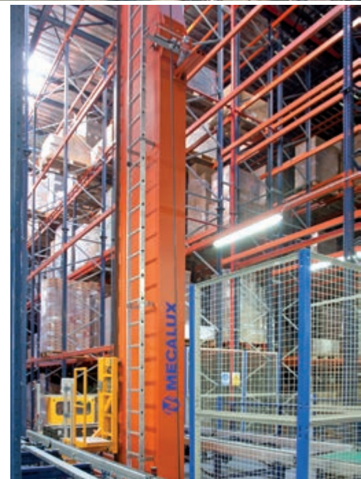
Automated warehouse with double-depth racking (2).
